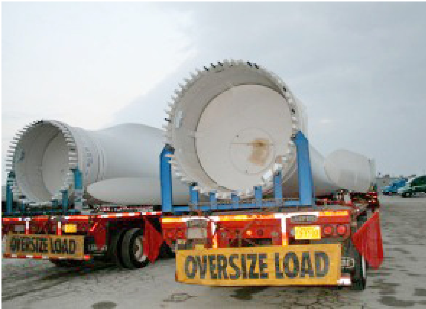
Wind turbine blades being transported to West Texas
